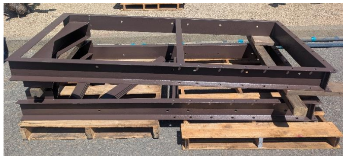
Figure 5: New gate frames
